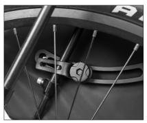
2. Clip the buckle into the bracket at an appropriate angle and fix it with a knob.
