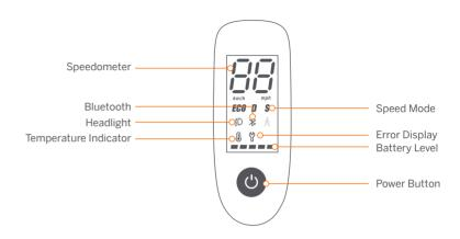
Power Button: Press the button to turn the KickScooter on and press, and hold the button for 3 seconds to turn the scooter off. When the KickScooter is on, press the button to turn on/off the headlight and the rear light, and press twice to switch between the speed modes.
