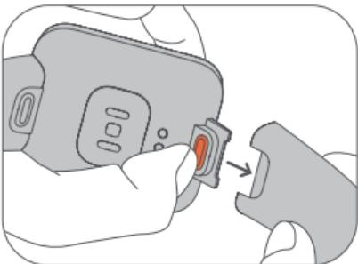
**Install the strap:** Align the slot of the strap with the watch and then insert it to the watch until you hear a click.
