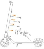
Install the external battery on the rail and fix it with the M4 (20mm) screws (2 pcs) and M3 screw (1 pcs), provided with this product. After they are properly installed, block the screw holes with the rubber stopper.
