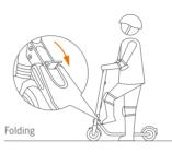
Step on the folding pedal while pushing the handlebar forward slightly.
