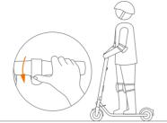
3. Put your other foot on the footrest to keep both feet stable. Press the throttle on right hand to speed up when you are balanced. Note: For your safety, the motor will not engage until the scooter reachs 2.5 mph (4 km/h)
