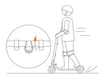
4. Slow down by releasing the throttle. Squeeze the electronic brake and stamp the fender with foot at the same time for a sudden brake
