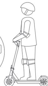
3. Put your other foot on the footrest to keep both feet stable. Press the throttle on the right hand to speed up when you are balanced.
