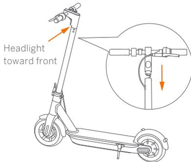
3. Install six screws (two on each side) with the included hex wrench.
