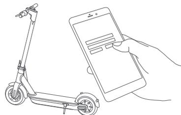
2 Power on the KickScooter. A blinking Bluetooth icon indicates the KickScooter is waiting for a connection.
