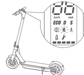
3 Click "Vehicle" → "Scan for Vehicle" to connect to your KickScooter. The KickScooter will beep when the connection is successful. The Bluetooth icon will stop blinking and remain illuminated.
